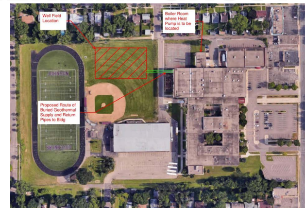
Site Photo Showing Location of Geothermal Well Field
